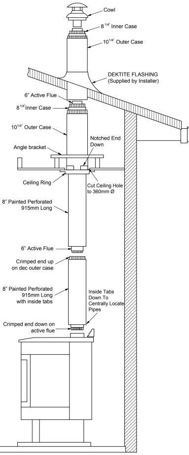
This flue kit has been manufactured in accordance with AS 2918:2018 and tested to appendix F.
